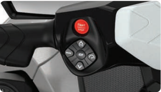
iDF – Intelligent Debris-Free Pump System (optional) An innovative, industry-first system that allows you to free your pump of weeds and debris with intuitive handlebar-activated controls.
