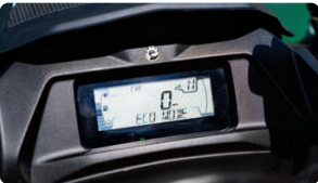
ECO® Mode This exclusive Sea-Doo® feature optimizes power output for up to 46% improved fuel efficiency.
