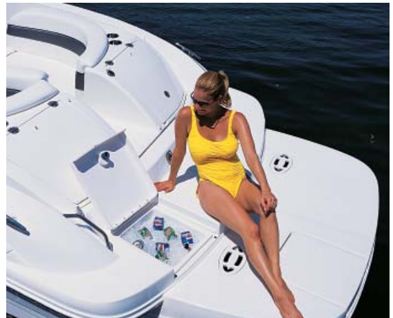
Standard integral swim platform features built-in cooler while optional extended swim platform includes concealed, stainless-steel ladder with integrated grab handle.
